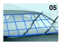
Apply just one layer of glass coating and allow it to dry for at least 6 hours.
