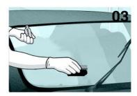
Work in cross-hatch pattern on small areas and make sure the coating is applied evenly.
