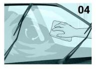
Let the product dry for 1 minute and remove excess residue using a 380gsm microfibre cloth. Inspect the surface thoroughly after wiping off to ensure there are no haze marks.
